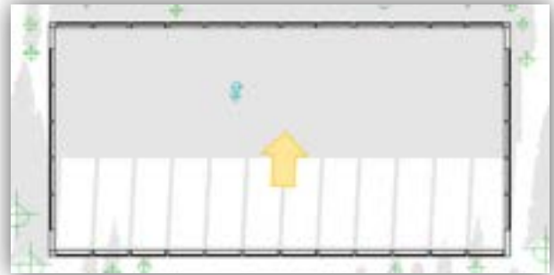
Figure 6: plan view at 3:00 PM (15:00) during an Equinox (March or September) with slab-to-slab windows and two-foot roof overhang. Source: primary.
