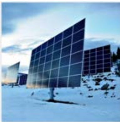
Figure 11 Dual Axis Tracker. Source: Deger Energie
