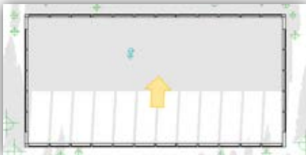
Figure 18: plan view at 3:00 PM (15:00) during an Equinox (March or September) with slab-to-slab windows and two-foot roof overhang. Source: primary.
