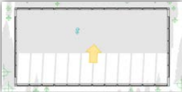
Figure 15: plan view at 3:00 PM (15:00) during an Equinox (March or September) with slab-to-slab windows and two-foot roof overhang. Source: primary.
