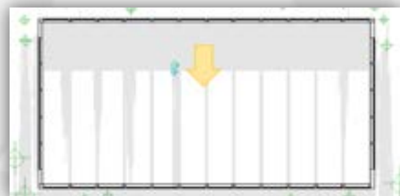
Figure 4: plan view at 3:00 AM on June 21 st (Summer Solstice) with slab-to-slab windows and two-foot roof overhang. Source: primary.
