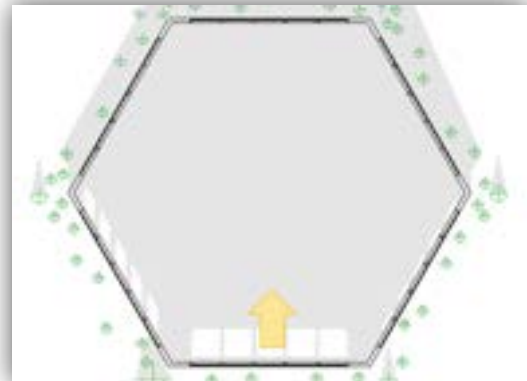
Figure 9: plan view at 3:00 PM (15:00) on June 21 st (Summer Solstice) with slab-to-slab windows and two-foot roof overhang. Source: primary.
